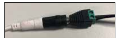
Wires connecting to charging port on Simplicity shade
